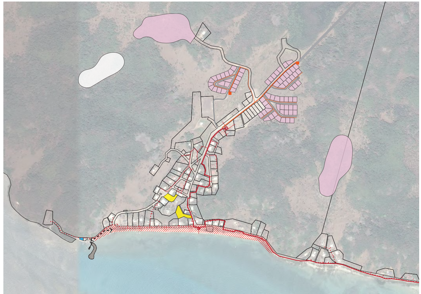
FIGURE 25: INFRASTRUCTURE REQUIREMENTS - SEWER
