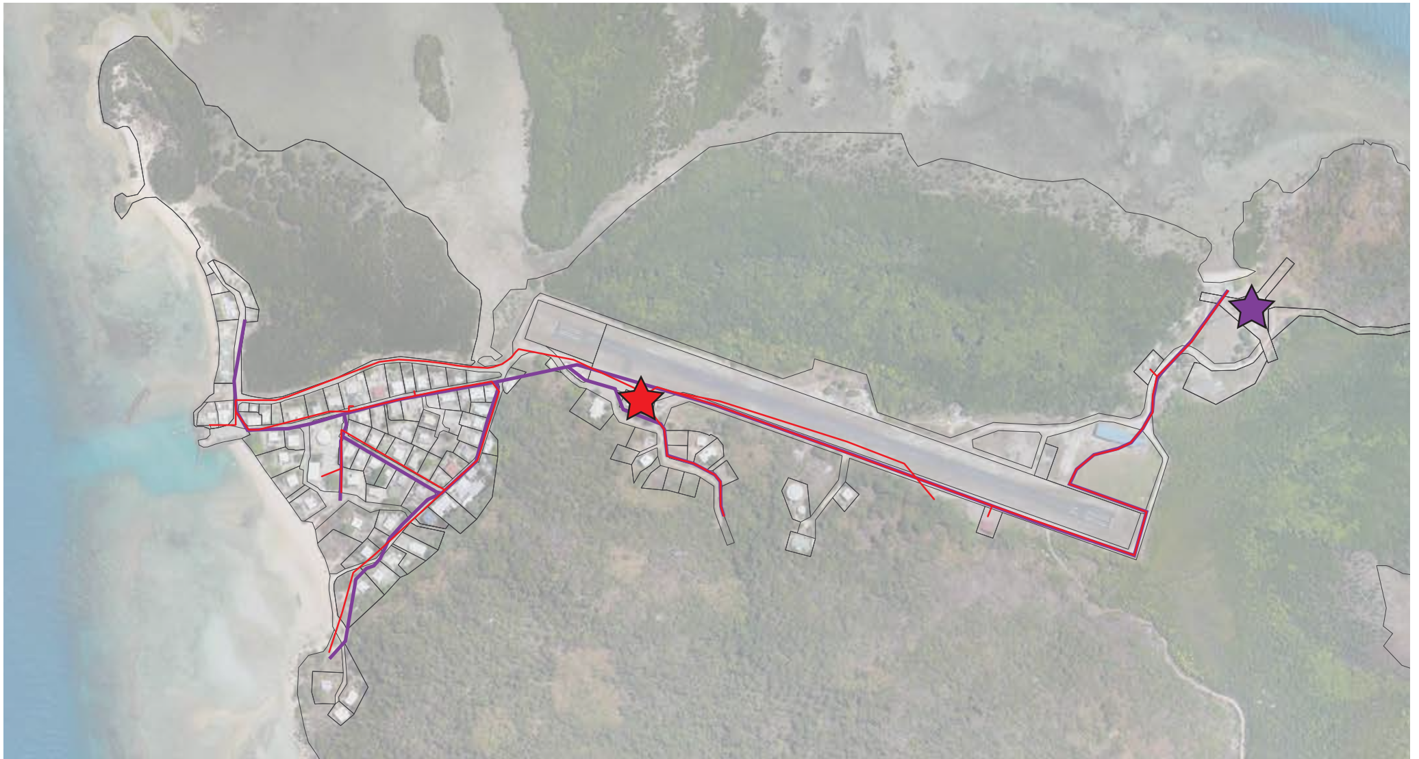
FIGURE 6: ELECTRICITY AND COMMUNICATIONS INFRASTRUCTURE - EXISTING
